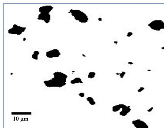
**Figure 4.** Optical microscope observation of roll milled pozzolana particles ( $\times 40$  magnification).
