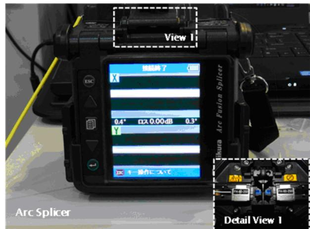
**Figure 11.** FBG connection setup and light bias test.
