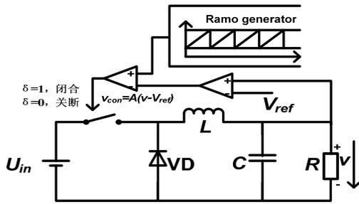
Figure 2 .Voltage type Buck converter.
