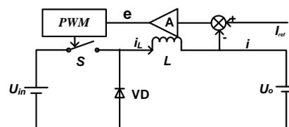
Figure 1. Current type Buck converter.
