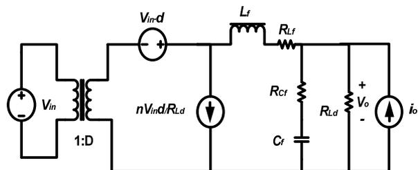
Figure 3. Buck converter small signal model.
