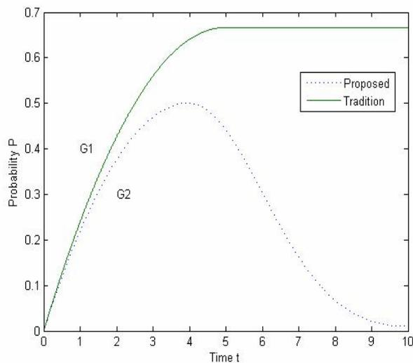
**Figure 4. Drop probability in traditional RED vs. proposed RED.**
