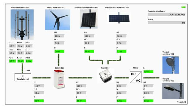
Figure 3. Visualization of the measured data with the help of the web interface.
