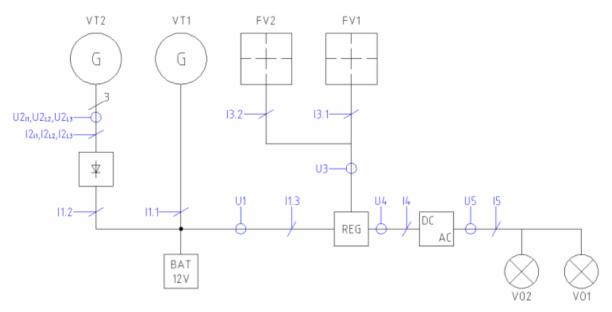
Figure 2. The block diagram of the measured system and the measuring points. [1]
