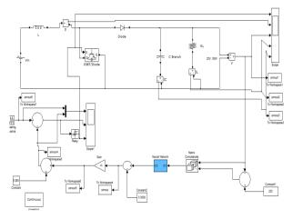
Figure 2. Simulink Model of Boost Converter.
