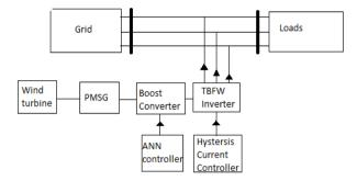
Figure 1. General Scheme of the Wind Energy Conversion System.
