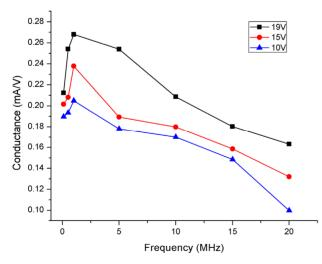
Figure 5. The conductance as a function of field frequency for three voltages (19 V, 15 V, and 10 V). A 1/64th concentration sample was sonicated for 30 minutes.
