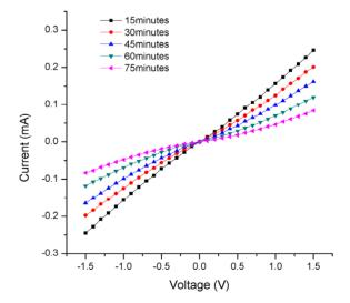
Figure 4. Plot of current vs voltage for a 1/64th concentration at different ultrasonication times. A 10 V peak-peak AC voltage was applied at a frequency of 15 MHz.
