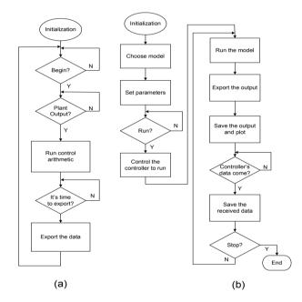
Figure 3. (a) Flow chart of the controller; (b) Flow chart in the simulating environment.
