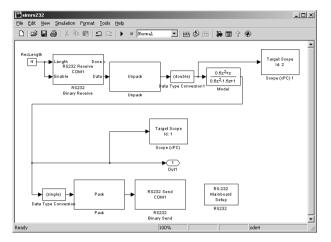
Figure 6. Simulink Diagram based on xPC Target.
