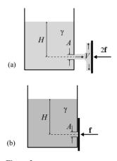
**Figure 3.** Dynamic (a) and static (b) forces of a fluid.
