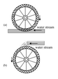
**Figure 1.** Examples of undershot wheel (a) and overshot wheel (b).
