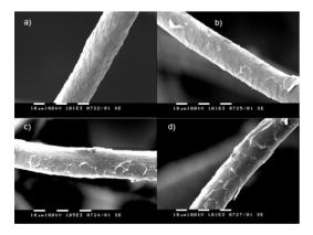
Figure 5. SEM microphotographs of the raw wool fibres after treatments with total enzyme concentration  $E_T$ : 6,5(mg/ml): (a / c) US combined Bioprot Multi / Bioprot Gentle, (b / d) Bioprot Multi / Bioprot Gentle.
