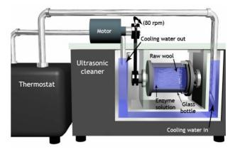
Figure 1. 3D plan view of the experimental equipment.
