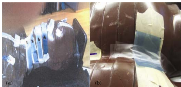
Figure 2. Geometrical setup for D_{\text{Surf}} measurements on Rando ® phantom.
