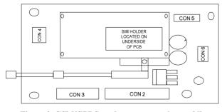
Figure 3. GSM/GPRS modem connector layout [4].
