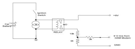
Figure 5. Ignition monitoring interfacing circuit.
