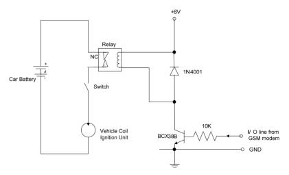
Figure 4. Demobilizer interfacing circuit.
