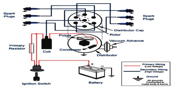
Figure 7. Coil ignition systems.
