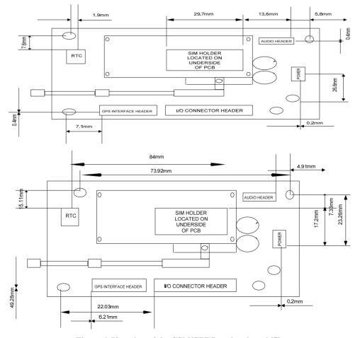
Figure 6. Plan view of the GSM/GPRS modem board [5].
