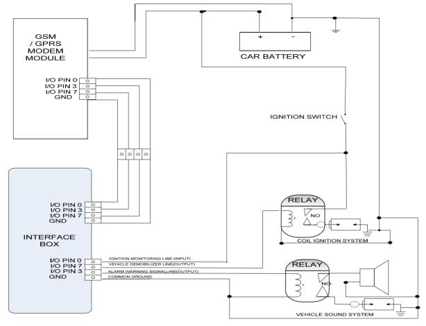
Figure 2. Wiring diagram of vehicle control subsystem.
