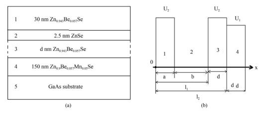
Figure 1. Nanoheterostructure, investigated in [1-3] (a) and its representation in space-energy diagram (b).
