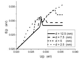
Figure 5. Electron ground state energy in the area of non monotony dependences for different width of unmagnetic layer.
