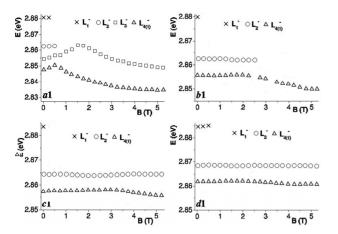
Figure 6. Magnetic field dependences of the energy positions of the Lorentz components for  $\sigma^-$  polarizations taken from [1]; a1: at d = 0; b1: at d = 2.5 nm; c1: at d = 7.5 nm; d1: at d = 12.5 nm.
