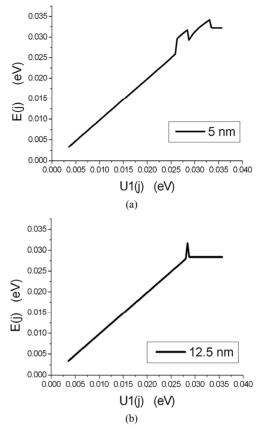
Figure 4. Ground state energy of electron as a function of potential  $U_1$ , changing in magnetic field because of Zeeman effect for different width of unmagnetic layer.
