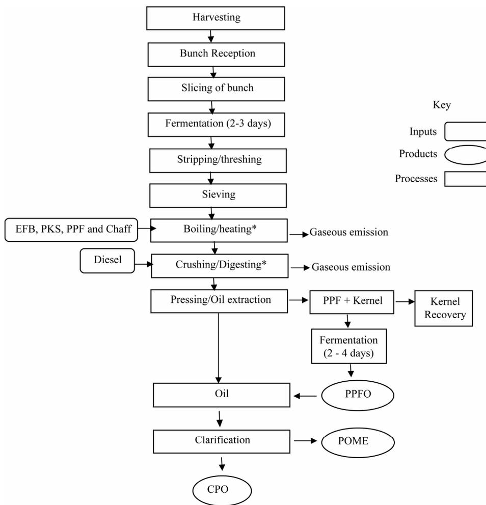
Figure 1. A schematic chart of palm oil processing by smallholders in Nigeria (\* = air quality sampling phase; POME = palm oil milling effluents; PPF = palm press fibre; PPFO = palm press fibre oil; CPO = crude palm oil).
