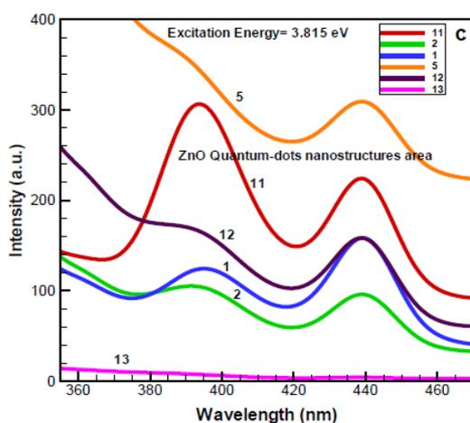
**Figure 12.** Photoluminescence spectroscopy of (c) some QDs ZnO nanoparticles (No. 11, 2, 1, 5, 12 and 13 from up to down respectively) between especial 360 - 460 nm wavelengths involving complex defects and expansion deep levels blue shift of products. They showed two different max peaks in two divers regions.
