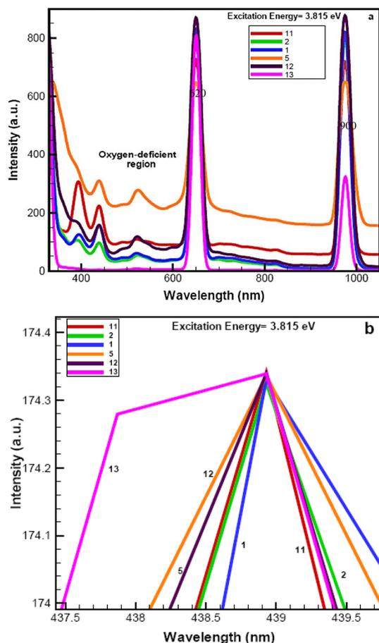
**Figure 11.** Photoluminescence spectra of (a) various QDs ZnO NPs and (b) the inset shows expansion of limited 437 - 439 nm wavelengths for illustration of broad, ladder and wave-like peaks of especial point defects. All of the products have 620 and 900 nm wavelength in (a) curve.
