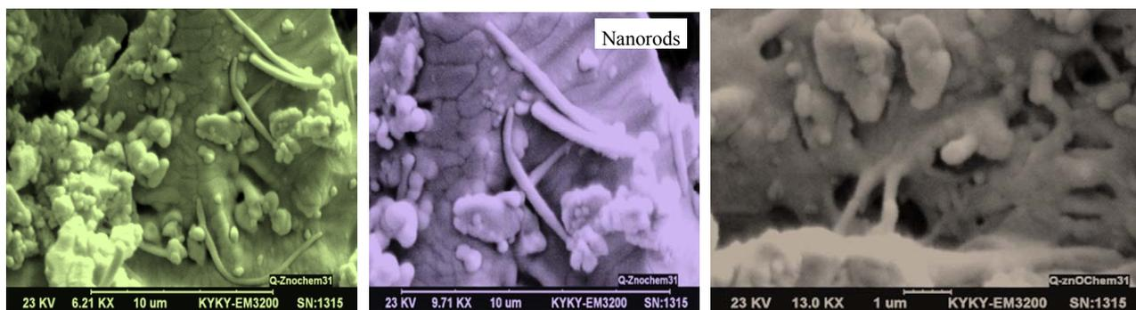
Figure 2. SEM images of QDs ZnO nanorods for sample 2.
