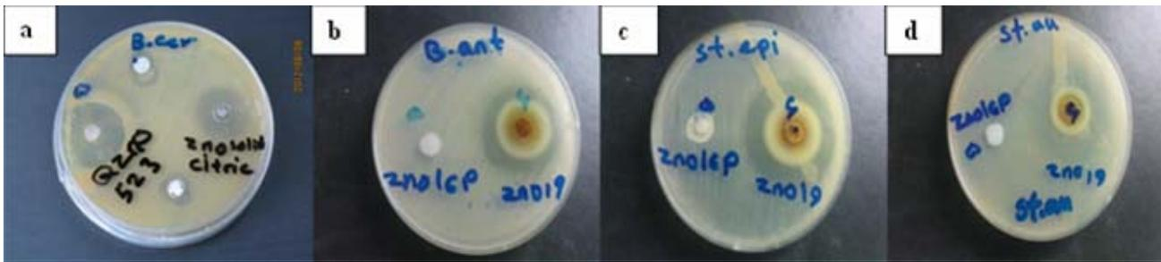
**Figure 13.** Agar plate test (well method) for (a) sample 5 (with symbol QZnO523) and (b)-(d) sample 8 (with symbol QZnO19) films showing excellent inhibition zone around the films. ZnO16P symbol is the same as sample 8 with polystyrene-capped which it was not successful during the growth process in well test.
