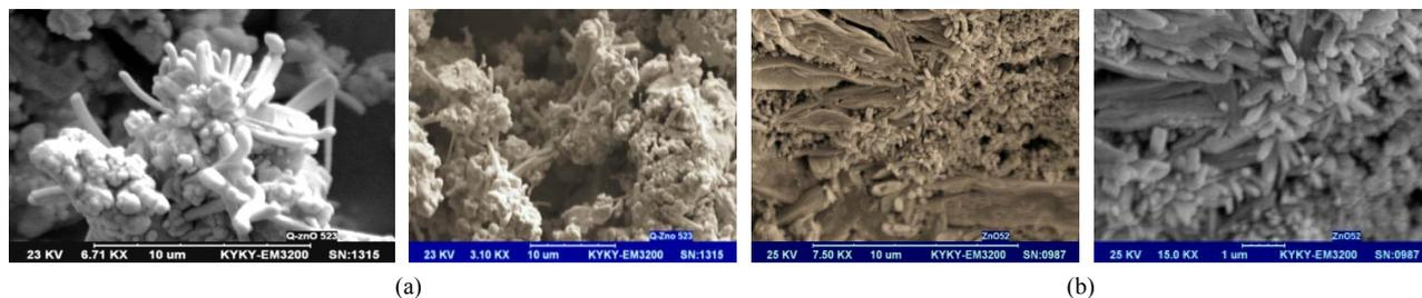
Figure 4. SEM images of nice formation of QDs ZnO nanorods for (a) sample 5 and (b) nanorods-nanoflowers mixture sample 13.
