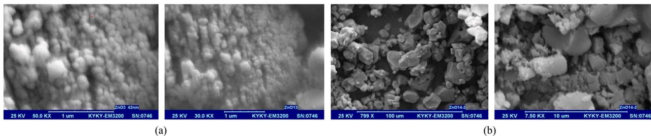
Figure 5. SEM images of two ZnO nanoparticles for (a) homogeneous of sample 6 and (b) sample 7.
