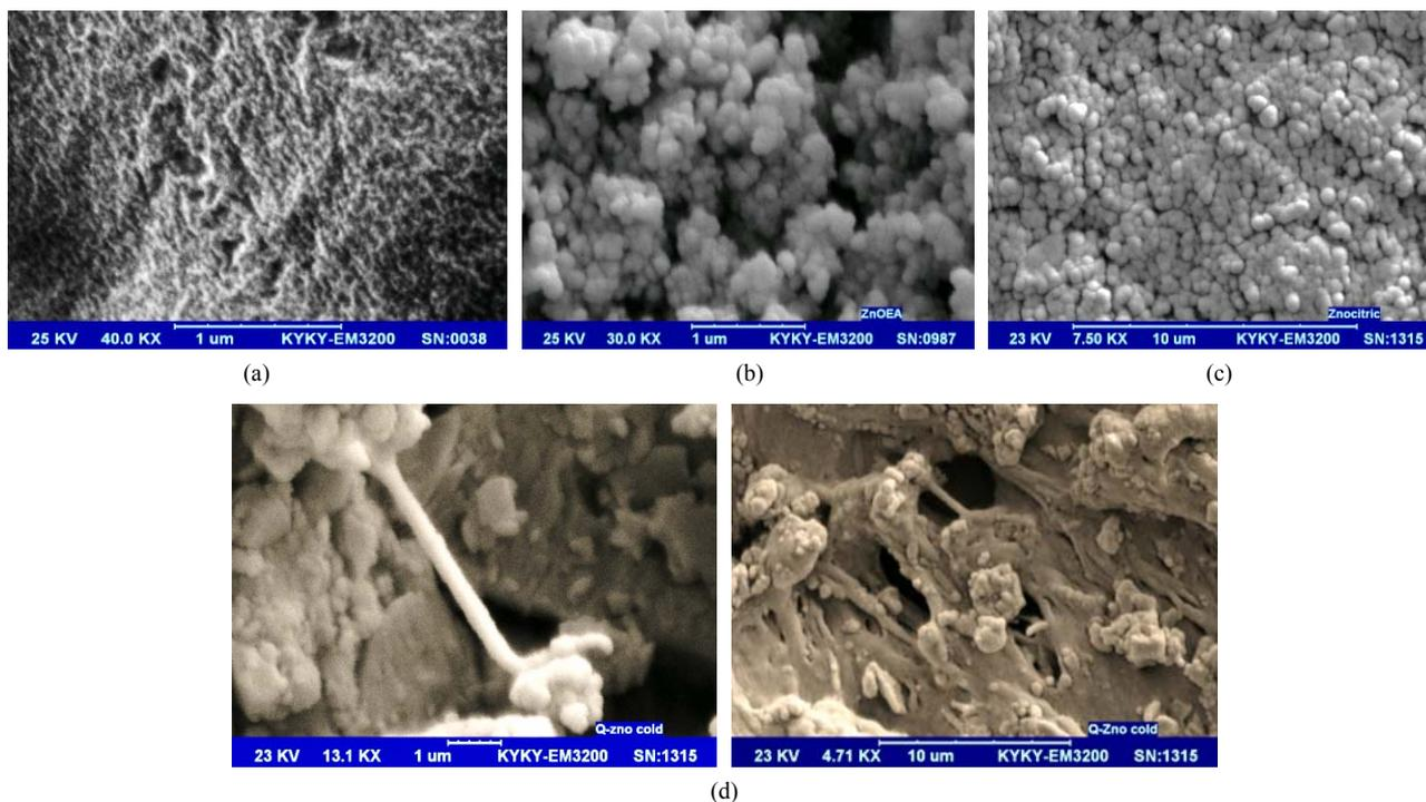
Figure 6. SEM images of various ZnO nanostructures for (a) ZnO QDs of sample 8; (b) sample 10; (c) sample 11 and (d) ZnO QDs as nanorods (nanotubes) for sample 12.
