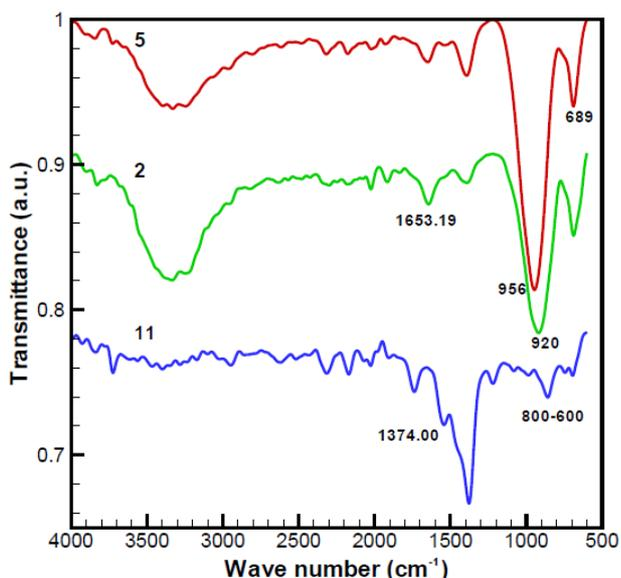
Figure 8. FTIR spectra of three ZnO nanoparticles for nanorods of samples 5 and 2 and nanospherical of sample 11 respectively.
