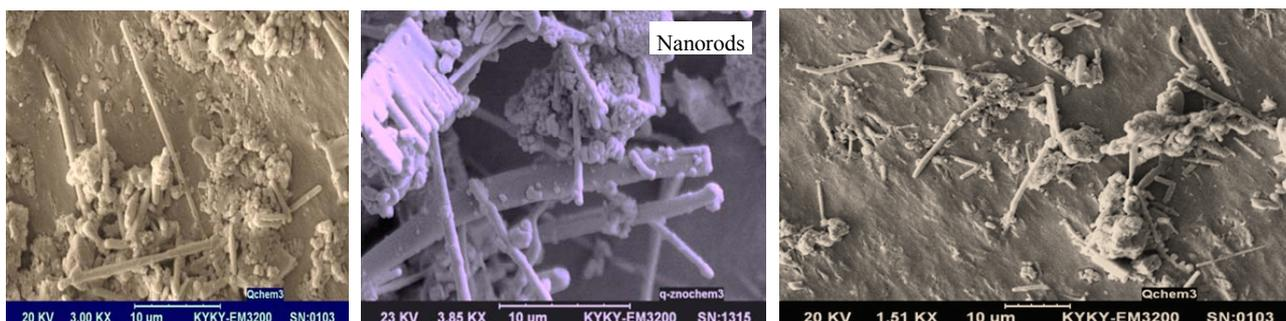
Figure 1. SEM images of QDs ZnO nanorods for sample 1.
