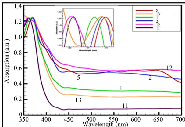
Figure 9. Optical absorption spectra of various QDs ZnO nanorods (samples 5, 13, 2, 12) and nanosphericals (samples 3, 11).
