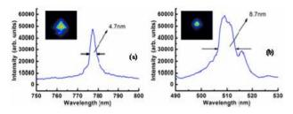
Figure 3. (a) SH spectra and mode; (b) TH spectra and mode.
