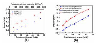
Figure 2. (a) Measured SH and TH power versus fundamental power; (b) SH and TH power including losses and fitting curves.
