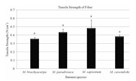
Figure 4. Fiber's tensile strength of *M. brachycarpa*, *M. paradisiaca*, *M. sapientum*, and *M. cavendishi*. Note: same notation that followed species showed not significantly different in Duncan  $\alpha$  0.05 test.
