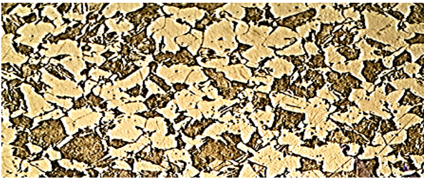
Plate 1. Microstructure of as-received steel sample showing pearlite (dark) in the matrix of ferrite (white). Etchant: 2% Nital. \times 400 .
