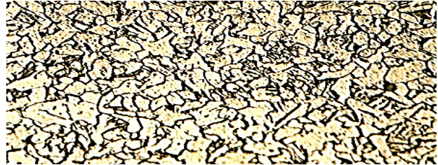
Plate 4. Microstructure of a sample of the carbon steel tempered at 200^{\circ}\text{C} for 1 hour showing tempered martensite. Etchant: 2% Nital. \times 400 .
