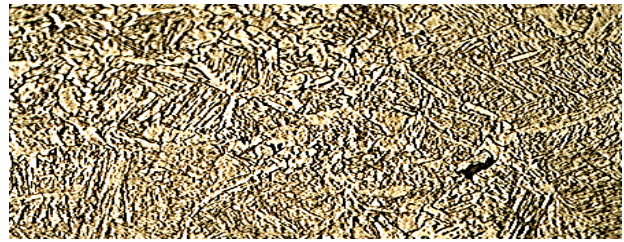
Plate 3. Microstructure of a water quenched sample showing martensite. Etchant: 2% Nital. \times 400 .
