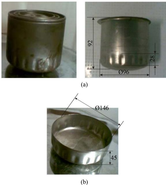
**Figure 6. Filter Casing Blanks Produced with New Method.**
