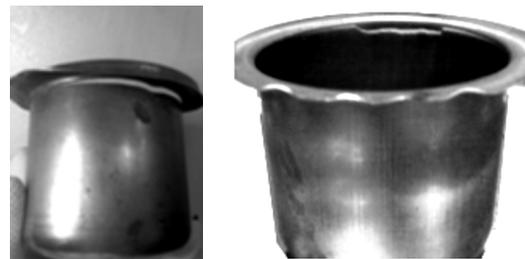
**Figure 4. Blanks with Cracks.**
