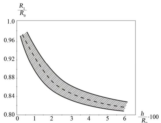
**Figure 3. Graph of Function  $\frac{R_1}{R_0} \left(\frac{h}{R_0}\right)$ .**
