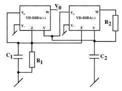
Figure 2. The proposed fully-uncoupled electronically controllable sinusoidal oscillator.
