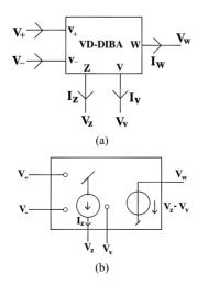
Figure 1. (a) Schematic symbol; (b) Behavioral model of VD-DIBA.
