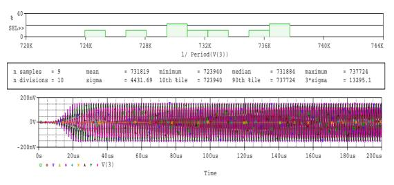
Figure 4. Result of Monte-Carlo simulation of oscillator circuit of Figure 2.
