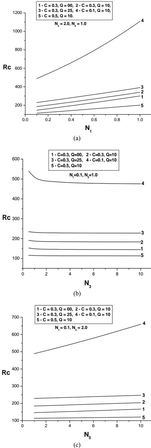
**Figure 7.** Plot of critical Rayleigh number  $R_c$  Vs. (a) coupling parameter  $N_1$ , (b) couple stress parameter  $N_3$ , (c) coupling parameter  $N_5$  with respect to rigid-free adiabatic no spin boundary condition for different values Chandrasekhar number  $Q$  and different values of Cattaneo number  $C$ .
