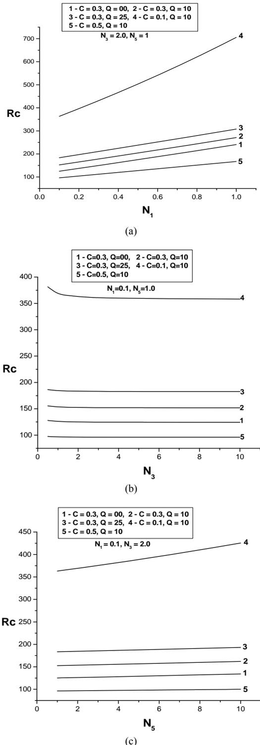
**Figure 2.** Plot of critical Rayleigh number  $R_c$  Vs. (a) coupling parameter  $N_1$ , (b) couple stress parameter  $N_3$ , (c) coupling parameter  $N_5$  with respect to free-free isothermal no spin boundary condition for different values Chandrasekhar number  $Q$  and different values of Cattaneo number  $C$ .
