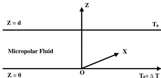
**Figure 1. Schematic diagram of the Rayleigh-Bénard situation for micropolar fluid.**
