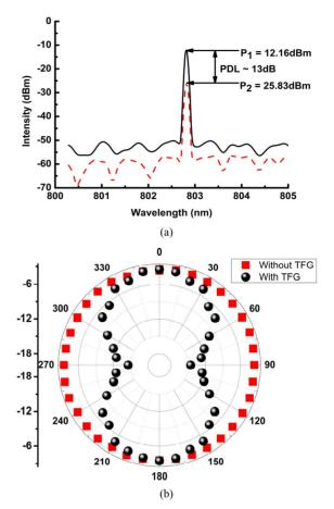
Figure 2. (a) The PDL measurement of S- and P-polarized light from the 15 mm long  $45^{\circ}$ -TFG, showing a PDL of ~13 dB; (b) Polarization distribution figure: Red square dots showing 0 dB PDL as measured from a virgin fiber; Black circle dots showing a near-8 figure shape measured from the 15 mm long  $45^{\circ}$ -TFG.
