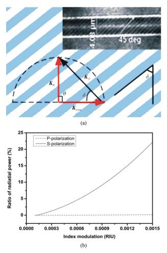
Figure 1. (a) Vector phase matching condition for a  $45^{\circ}$ -TFG; Inset: microscopic image of a UV-inscribed  $45^{\circ}$ -TFG; (b) simulated ratio of radiation power of *S*- (solid line) and *P*-polarization (dash line) for a  $45^{\circ}$ -TFG.
