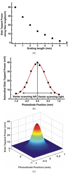
Figure 4. (a) Measured side-tapped out power along the length for the 9 mm 45'-TFG; (b) Measured power distribution in azimuthal direction, showing a Gaussian profile; (c) Replotted measured power distribution in azimuthal direction in 3-D.
