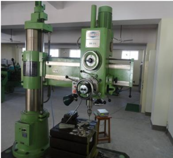
Figure 1. Drilling machine showing the dynamometer used for measurement of cutting forces.
