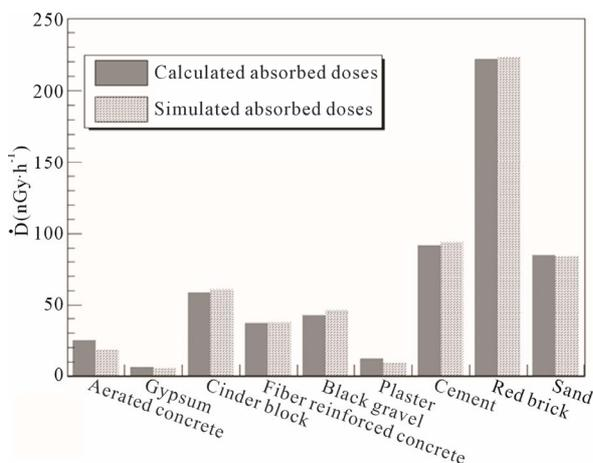
Figure 7. Comparison between the calculated and simulated absorbed doses.
