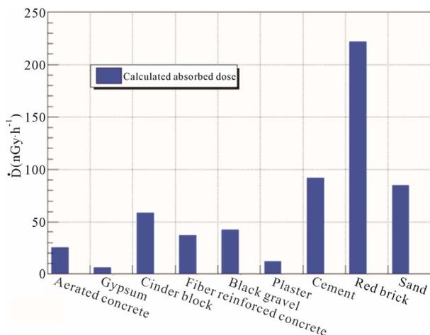
**Figure 3.** The absorbed dose  $\dot{D}$  according to the room model of UNSCEAR.
