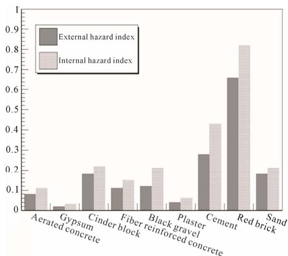
**Figure 2.** External and internal indexes calculated according to the models of Equations (1) and (2).
