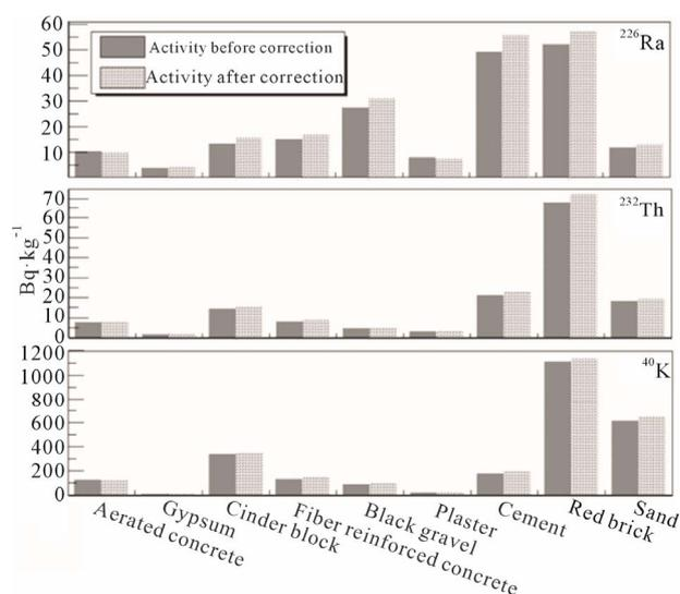
**Figure 1.** Specific natural radioactivity of the nine building materials without and with corrections for coincidence summing and self-absorption.
