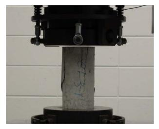
Figure 3. Compressive strength test.
