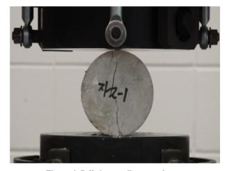
Figure 4. Splitting tensile strength test.
