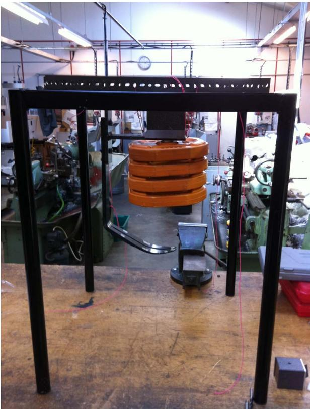
**Figure 5.** Prosthesis drop test rig.
