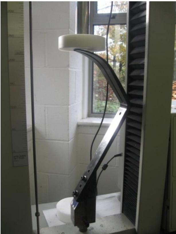
**Figure 3.** Prosthetic blade loading.
