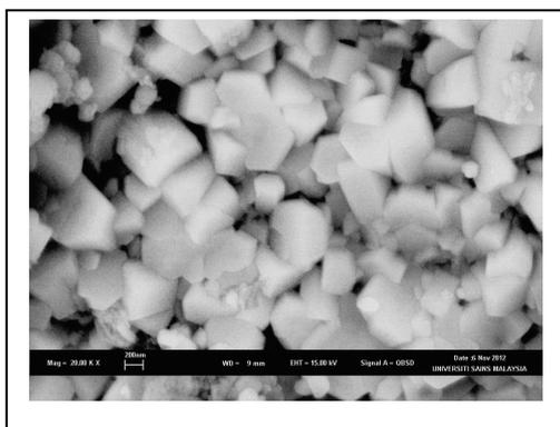
Figure 4. SEM micrograph of Sample 2 magnified 20000 times.
