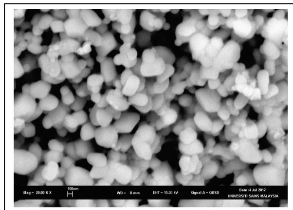
Figure 6. SEM micrograph of Sample 4 magnified 20000 times.
