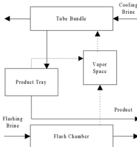
Figure 2. The structure of a single flash stage.
