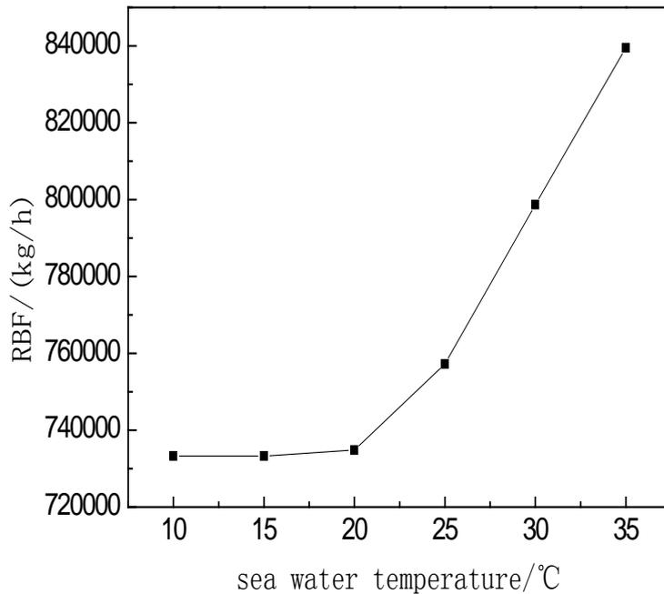
Figure 4. Effect of feed seawater temperature on the RBF.
