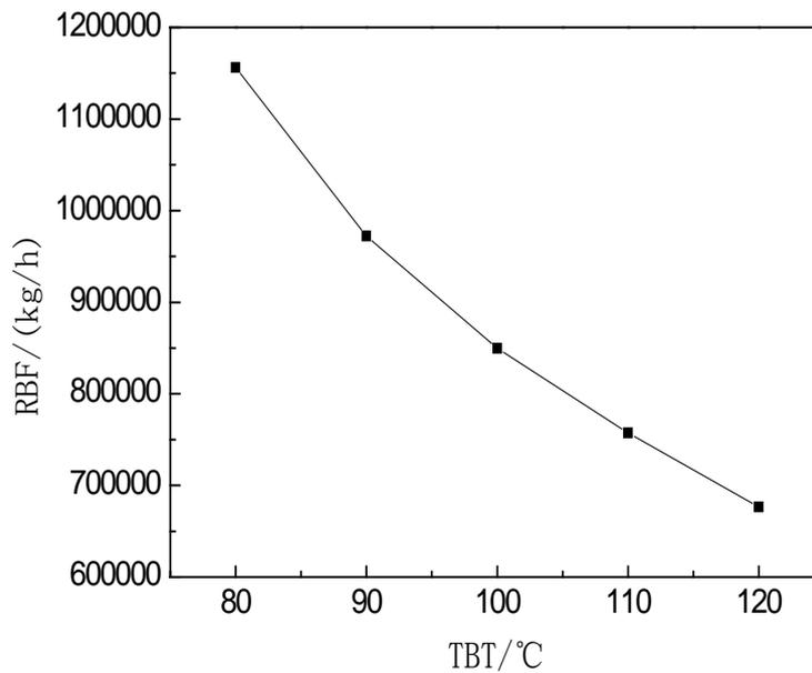
Figure 6. Effect of top brine temperature on the RBF.
