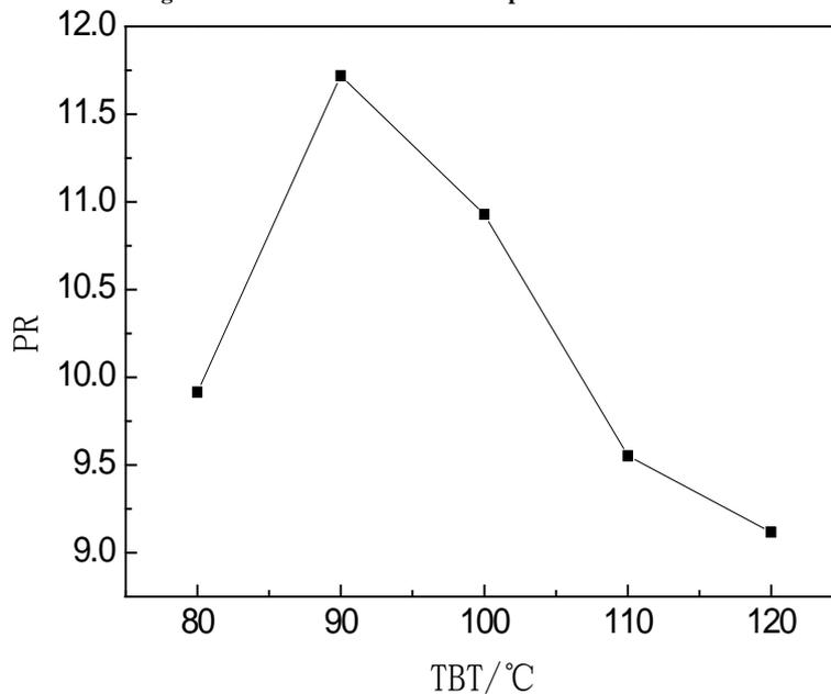
Figure 5. Effect of top brine temperature on the PR.
