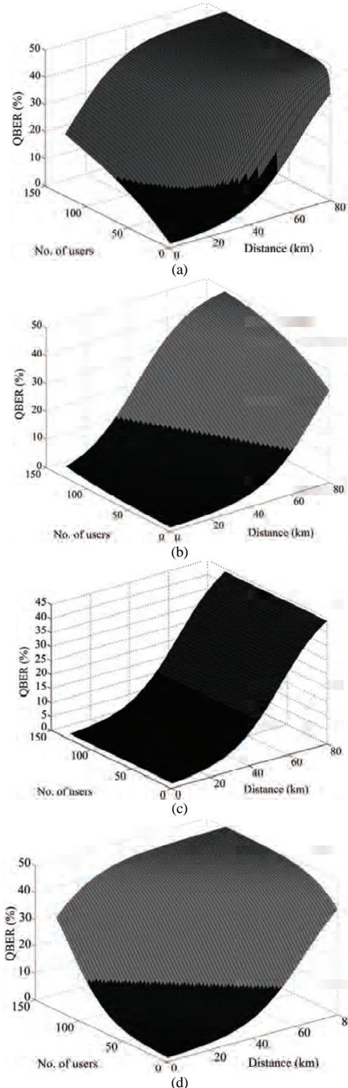
**Figure 10.** B92-protocol topologies at 1310 nm. QBER surface as a function of users and distance. Users range: 2-128 users. Distance range: 0- 80 km. QBER<14% in shaded region. (a) Passive Star B92 1310 nm; (b) Optical Ring B92 1310 nm; (c) Wavelength-routed B92 1310 nm; (d) Wavelength-addressed bus B92 1310 nm.
