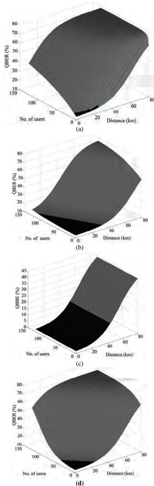
**Figure 13.** EPR- protocol, topologies at 1310 nm. QBER surface as a function of users and distance. Users range: 2-128 users. Distance range: 0-80 km. QBER < 15% in shaded region. (a) Passive Star EPR 1310 nm; (b) Optical Ring EPR 1310 nm; (c) Wavelength-routed EPR 1310 nm; (d) Wavelength-addressed bus EPR 1310 nm.
