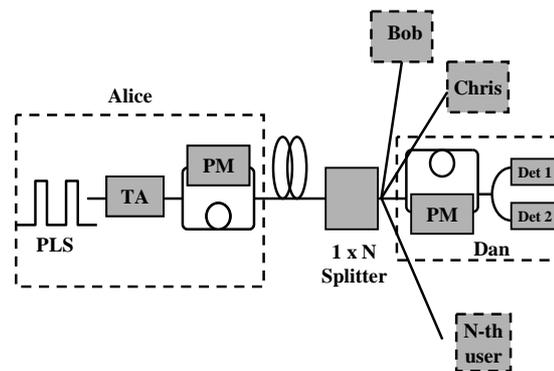
Figure 3. Network topology of passive-star multi-user QKD network. (PLS: Pulsed laser source; TA: tunable attenuator; PM: phase modulator; Det: detector.).
