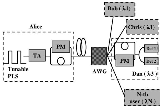
Figure 5. Network topology of wavelength-routed multi-user QKD network. (AWG: arrayed-waveguide grating).
