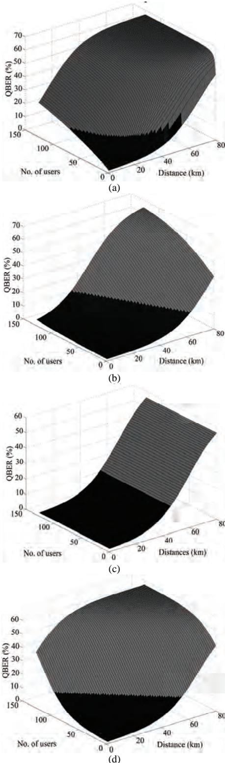
Figures 12. SSP, topologies at 1310 nm. QBER surface as a function of users and distance. Users range: 2-128 users. Distance range: 0- 80 km. QBER<17% in shaded region. (a) Passive Star SSP 1310 nm; (b) Optical Ring SSP 1310 nm; (c) Wavelength-routed SSP 1310 nm; (d) Wavelength-addressed bus SSP 1310 nm.
