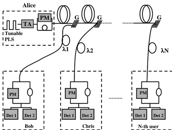
Figure 6. Network topology of wavelength-addressed bus multi-user QKD network. (G: fibre Bragg grating).
