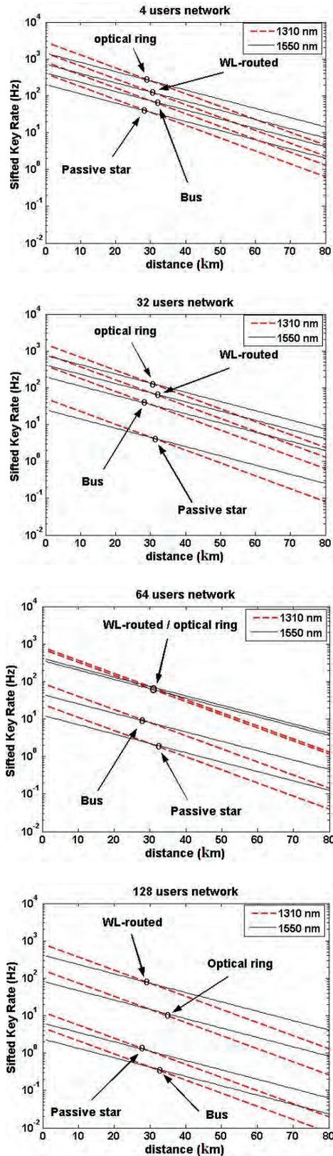
Figure 17. EPR-protocol. Sifted Key Rate versus distance for 4, 32, 64, 128 users.
