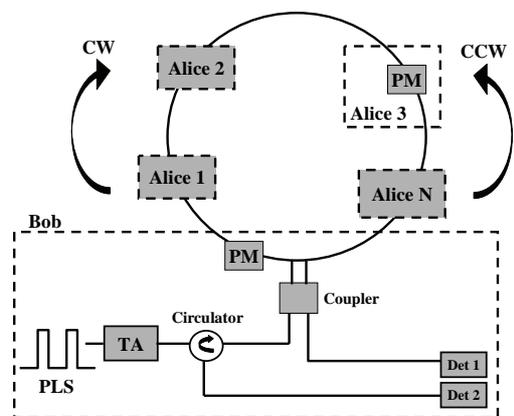
Figure 4. Network topology of optical-ring multi-user QKD network based on Signac interferometer.
