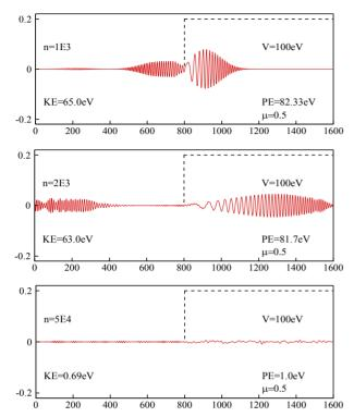
Figure 4. Simulation of an electron moving in free space and then hitting a potential. The second-order FDTD scheme was employed with  $\mu=0.5$  and absorbing boundary condition.
