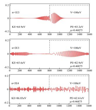
Figure 1. Simulation of an electron moving in free space and then hitting a potential. The original FDTD-Q scheme was employed with  $\mu=0.46875$  and no absorbing boundary condition. Here, the horizontal coordinate is k and the vertical coordinate is  $\psi_{\rm real}$ .
