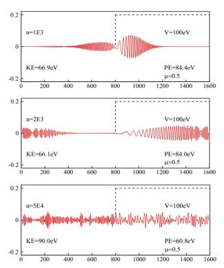
Figure 5. Simulation of an electron moving in free space and then hitting a potential. The fourth-order FDTD scheme was employed with  $\mu=0.5$  and no absorbing boundary condition.
