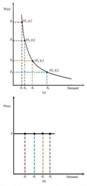
Figure 1. (a) Demand and price curve for optional (variable) loads; (b) Demand and price curve for fixed (must run) loads.
