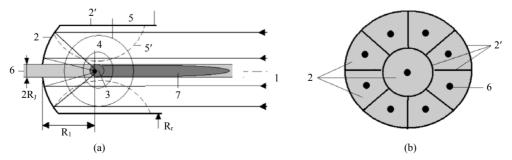
**Figure 1.** Scheme of reflector (a) and possible structure of matrix of reflectors (b) for LJE. 1: high rep. rate P-P laser radiation; 2: back side of reflector-zone of laser pulses interaction; 2': side wall of reflector; 3: cavern; 4: OPD; 5: shock wave; 5': reflected shock wave; 6: gas stream; 7: plasma stream.
