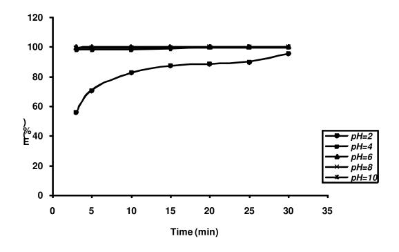
Fig.6:Temporal coag-flocculation efficiency profile at 300mg/l and pH varying CWE.
