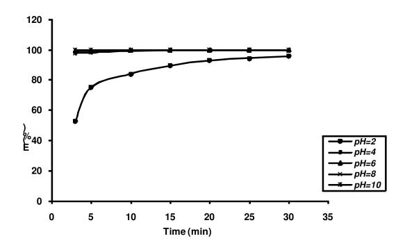
Fig.7 :Temporal coag-flocculation efficiency profile at 400mg/l and pH varying CWE.
