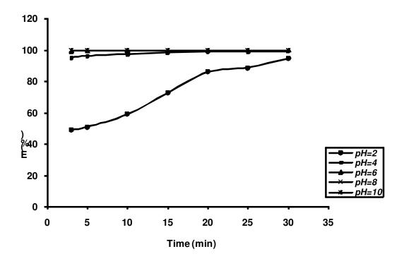
Fig.5: Temporal coag-flocculation efficiency profile at 200mg/l and pH varying CWE
