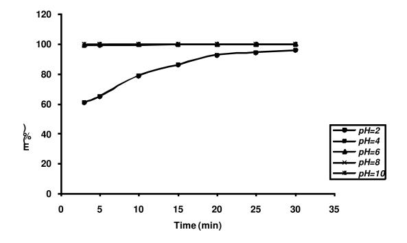
Fig.8: Temporal coag-flocculation efficiency profile at 500mg/l and pH varying CWE.
