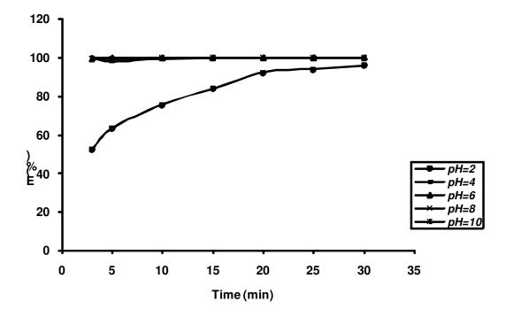
Fig. 4: Temporal coag-flocculation efficiency profile at 100mg/l and pH varying CWE.
