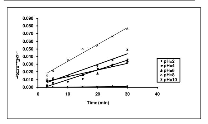
Fig. 1: Kinetic profile of SDP removal from CWE by CDC at 100mg/l
