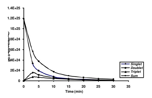
Fig.3:Temporal particle aggregation profile at maximum half life of 3.3825min
