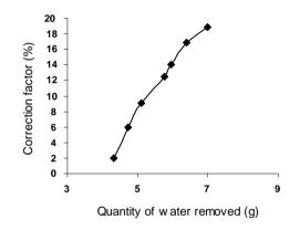
Fig. 6: Variation of model-predicted quantity of water removed with its associated correction factor
