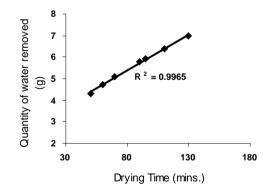
Fig. 2: Variation of the quantity of water evaporated with drying time (as predicted by derived model)
