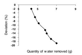
Fig. 4: Variation of model-predicted quantity of water removed with its associated deviation from experimental result
