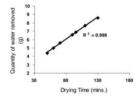
Fig.1: Variation of the quantity of water evaporated with drying time (as obtained from experiment)
