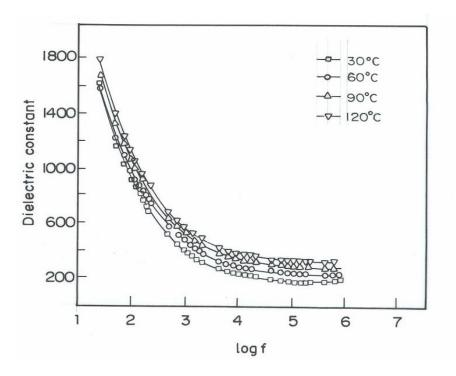
Fig. 5. Variation of dielectric constant with frequency
