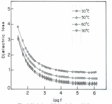
Fig. 6. Variation of dielectric loss with frequency
