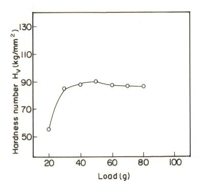
Fig. 4. Vickers microhardness number vs load
