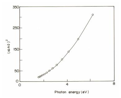
**Fig. 3** Plot of  $(\alpha h v)^2$  versus hv for GZC single crystal
