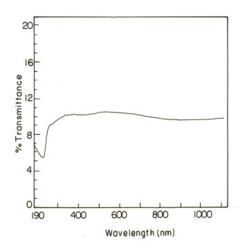
Fig. 2 UV-visible transmittance spectrum of GZC
