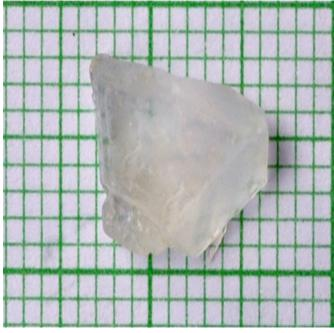
Fig. 1. As-grown single crystals of GZC
