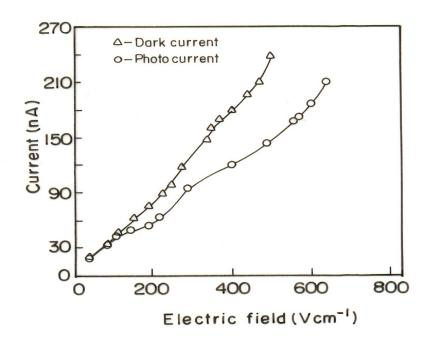
Fig. 7. Photoconductivity of grown crystals
