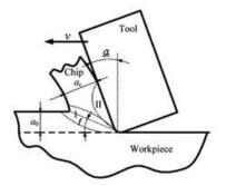
Fig.3 Schematic of plane strain machining with other parameters
