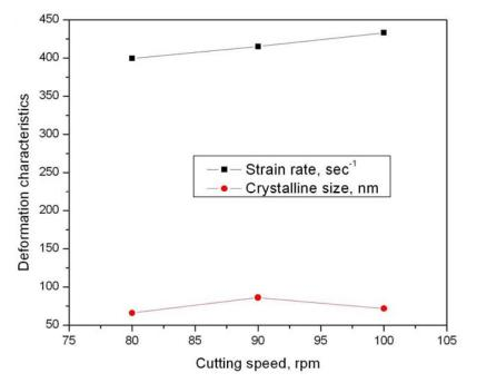
Fig. 4(b) Effect of cutting speed on strain rate and crystallite size
