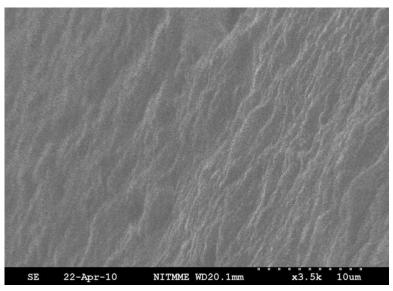
Fig. 1 SEM micrograph of Ultrafine grained chip after machining
