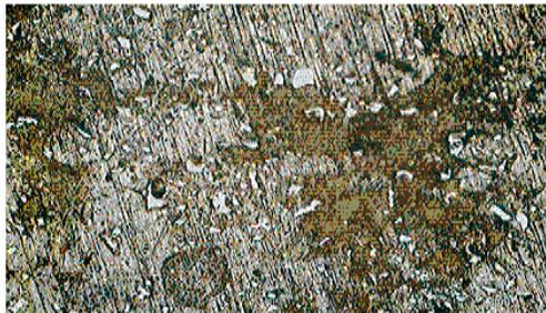
Micrograph 6: Tin tailings with (25% Al-Si alloy). x200 with random white patches of  $\text{Al}_6\text{Si}$  particles in the ceramic phase (Black).
