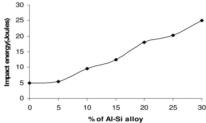
Fig 5: Variation of impact energy with percentage of Al-Si alloy addition.
