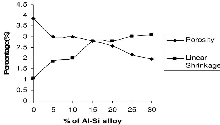
Fig 2: Variation of linear shrinkage and porosity with percentage addition Al-Si alloy Tensile Properties.
