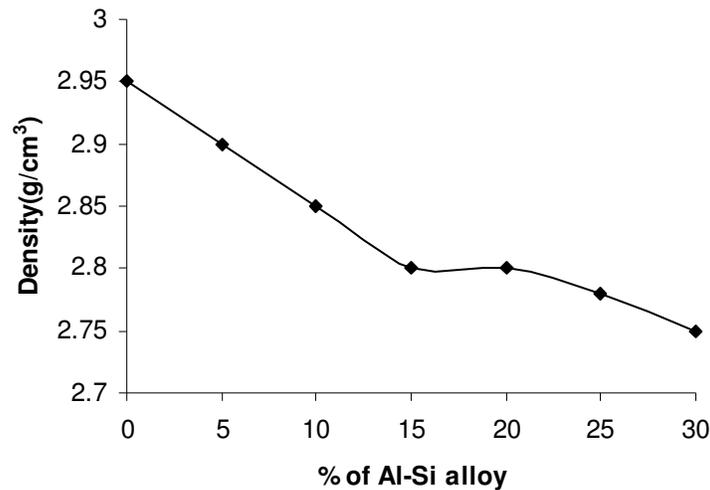
Fig 1: Variation of density with percentage addition of Al-6% Si alloy
