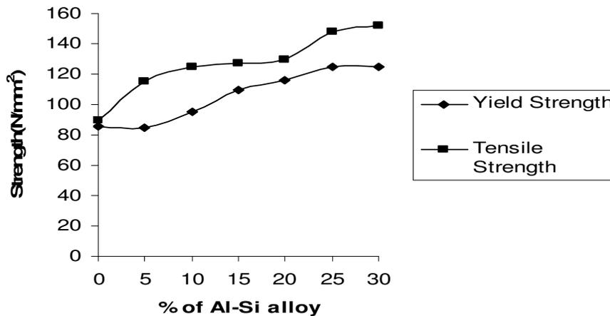
Fig 3: Variation of yield and tensile strength with percentage of Al-Si alloy addition.
