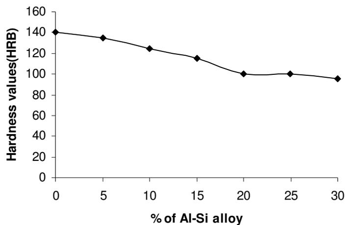
Fig 4: Variation of hardness with percentage addition of Al-Si alloy.
