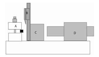
Figure 1. Diagram of the tissue-sectioning device. The osteochondral sample is held in the customized clamp (A). The single bevel-edged razor blade is able to move up and down to slice the 0.1 mm osteochondral slices (B). C shows the movable metal block holding the cutting apparatus. D is a digital micrometer (Parker Automation, UK) with an accuracy of 0.0001 mm that was used to move the blade towards the tissue sample.
