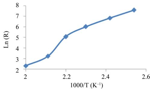
Figure 9. Arrhenius plot for the ZnO sensing element.
