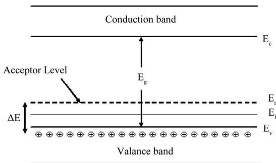
**Figure 8. Band diagram for activation energy in p-type semiconductor.**
