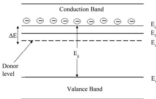
**Figure 7. Band diagram for activation energy in n-type semiconductor.**
