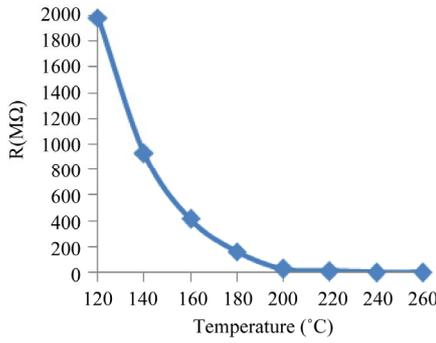
**Figure 5. Variations in resistance with temperatures of ZnO sensing element.**
