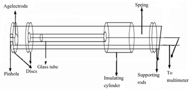
**Figure 4.** Sample holder (Ag-pellet-Ag electrode configuration).
