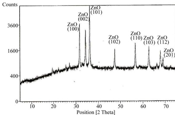
**Figure 2.** X-Ray diffraction of synthesized ZnO powder prepared at room temperature.
