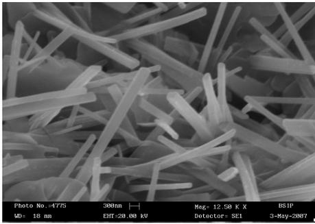
**Figure 1.** Scanning electron micrograph of ZnO in the form of pellet.
