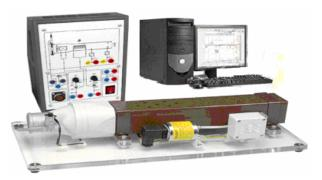
Figure 2. Three-dimensional view of aerothermic process.
