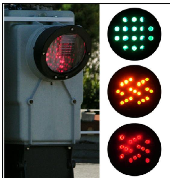
**Figure 1.** Typical Italian railway signal and example of LED matrix for different color aspects.
