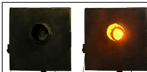
**Figure 2.** Thermal chamber built to test railway signals.
