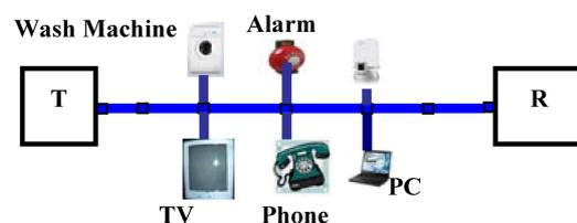
Figure 1. Model of a PLC network.
