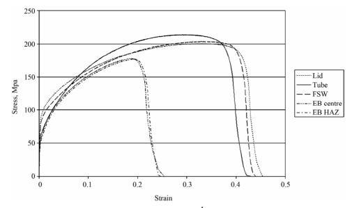
Figure 2. Stress-strain curves of test samples tested at strain rate  $10^{-4}$  1/s. Tensile strength of the EB weld is low compared to that of the other samples, 175 MPa as compared to 200 MPa or higher and the uniform elongation is about half of that of the FSW weld and the lid and tube base materials.
