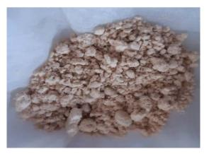
Figure 2. CMC from garments wastes (after final step).
