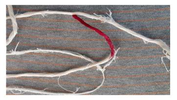
Figure 8. Newly sized yarn after absorbency test.
