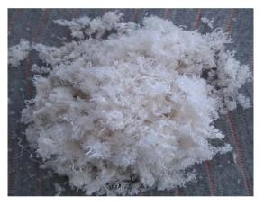
Figure 1. Sliced fabric wastages (after first step).
