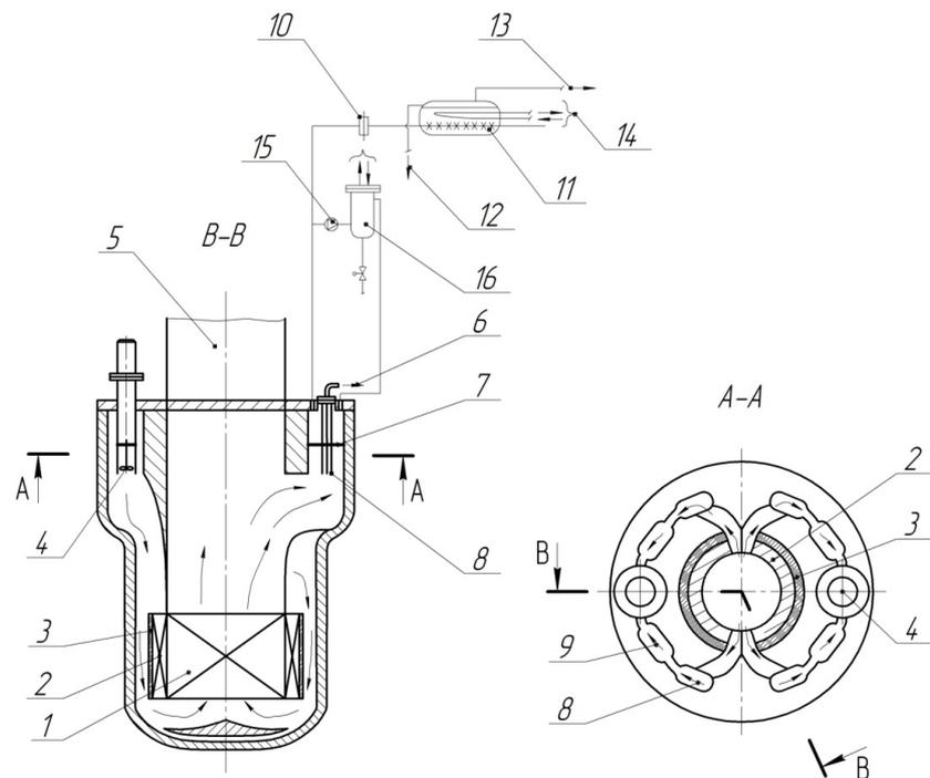
1—reactor core; 2—neutron reflector; 3—biological protection; 4—main circulation pump; 5—reactor control and protection system rods; 6—superheated steam line to turbine; 7—free HLMC level; 8—steam generator superheater; 9—steam generator evaporator; 10—burst diaphragm; 11—relief tank; 12—condensate to special water treatment system; 13—gas to gas treatment system; 14—cooling water; 15—gas circulator; 16—safety steam condenser.
