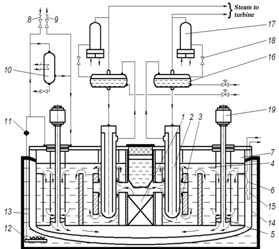
1—reactor core; 2—steam generator; 3—steam generator sub-header; 4—steam generator top header; 5—main circulation pump; 6—free coolant level; 7—unit gas plenum; 8—gas supply pipeline; 9—gas discharge pipeline; 10— isolation condenser; 11—burst diaphragm; 12—sparger; 13—water region of passive heat-rejection system tank; 14—guard vessel; 15—steam heating equipment; 16—separator; 17—cooling condenser; 18—shut-off control valve; 19—pump motor.
