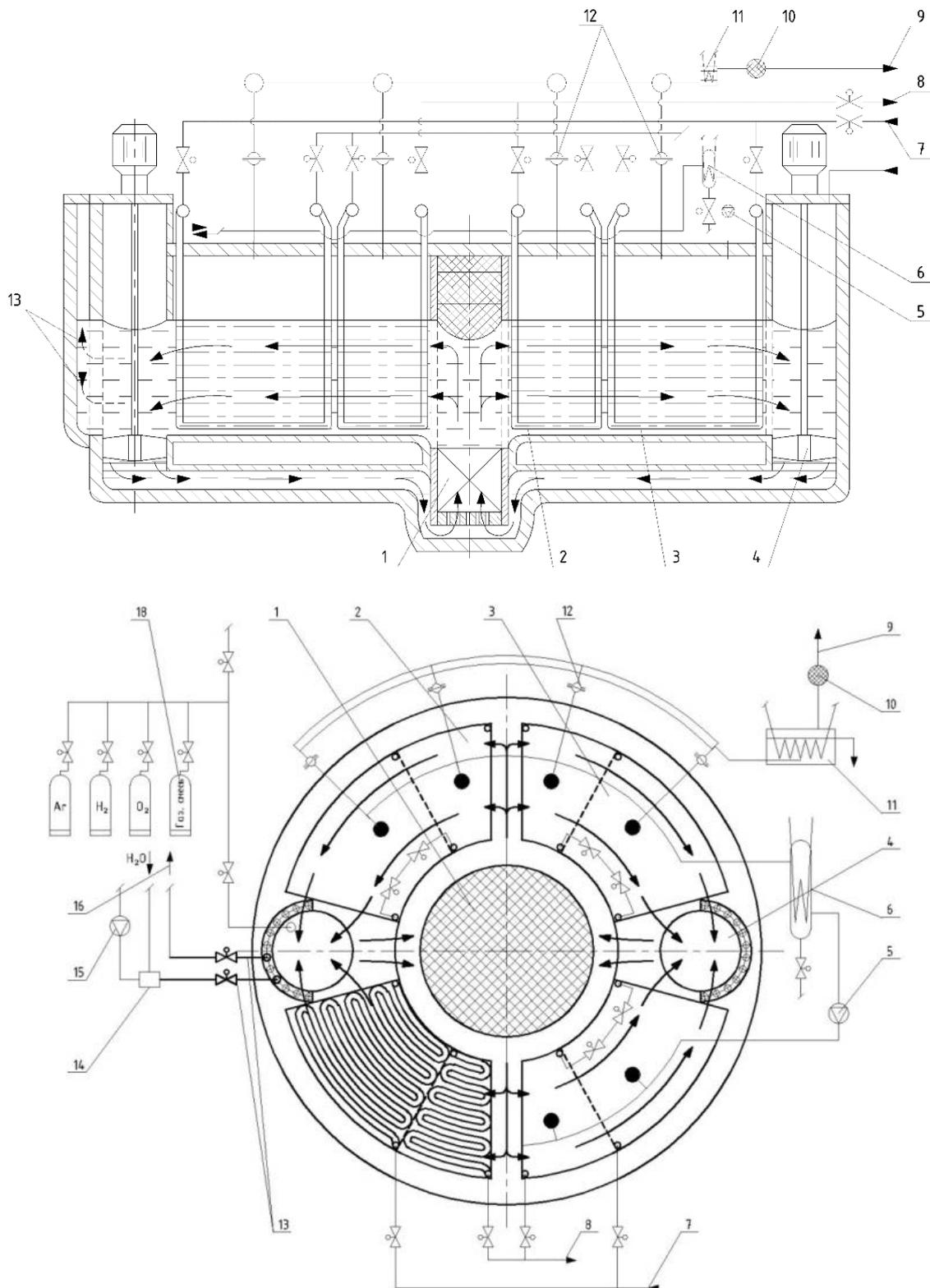
1—reactor core; 2—steam superheater; 3—evaporator; 4—main circulation pump; 5—gas circulator; 6— isolation condenser; 7— feed water supply; 8—steam to turbine; 9—gas blow-off line; 10—filter; 11—condenser; 12—burst diaphragm; 13—to standby and emergency heat removal system; 14—mixer; 15—compressor; 16—air-steam mixture outlet
