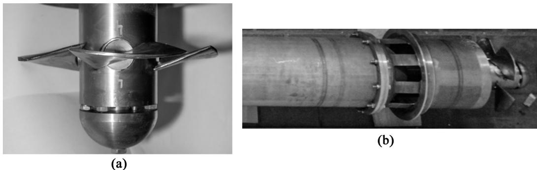
**Figure 5.** Pictures of (a) Shaft-Mounted Impeller and (b) Main View of Pump with Rotating Blades.
