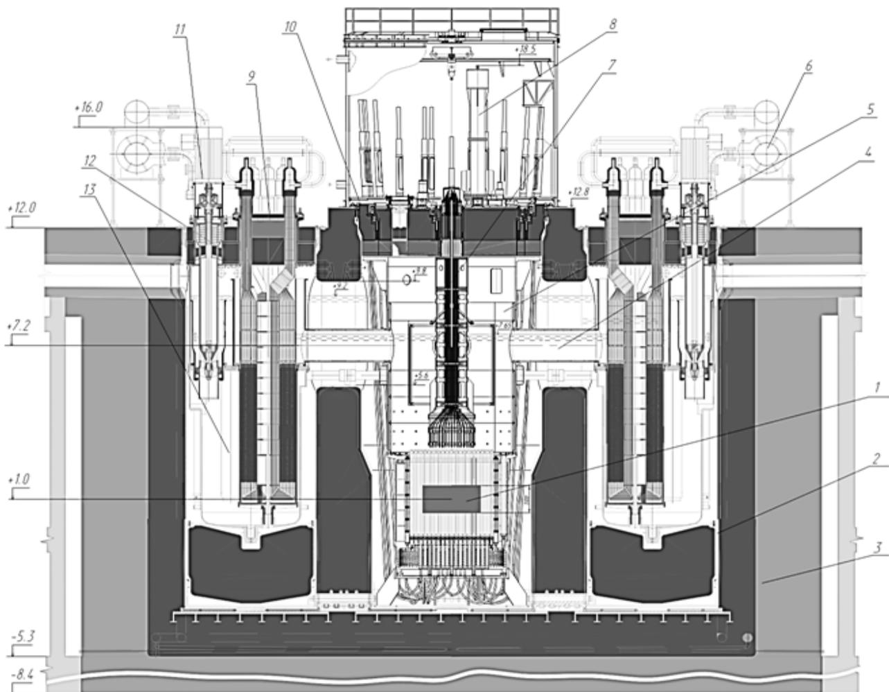
1. Reactor core; 2. Casing unit; 3. Reactor pit; 4. Header pipeline; 5. Reactor core barrel; 6. Cooldown system; 7. Measuring column; 8. In-vessel transfer machine; 9. Steam generator; 10. Top covering; 11. Main circulation pump; 12. Steam generator-MCP unit; 13. Filter.
