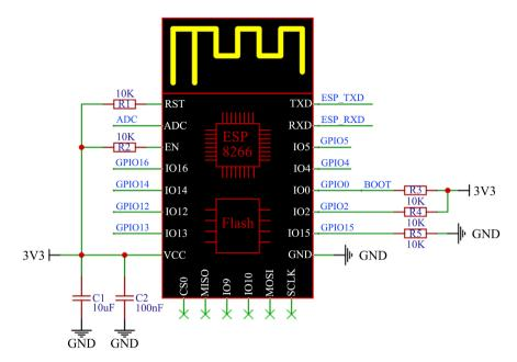
Figure 4. Minimal system circuit diagram.
