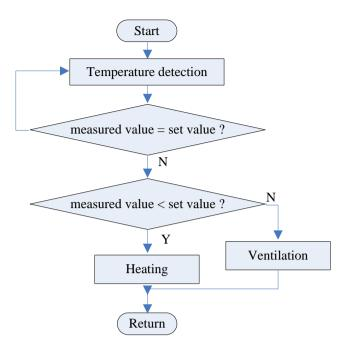
Figure 3. Temperature detection control flow chart.
