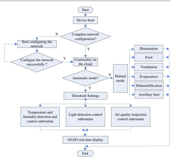
Figure 2. Main flow chart of system control.
