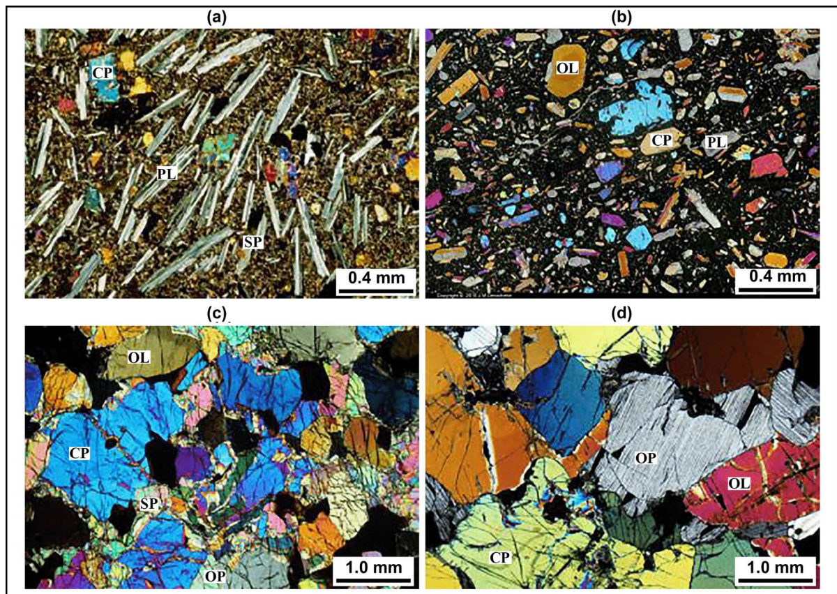
Figure 3. Photomicrographs of GPVF thin sections. (a) A basanite (Sample GS11— Table 3 ) from the Alwastani Mountain, (b) An alkali olivine basalt (Sample GS55— Table 3 ) from the Jesr Alshoguor area, (c) A lherzolite (Sample GX23— Table 4 ) from Jesr Alshoguor area, and (d) A harzburgite (Sample GX19— Table 4 ) from the Jesr Alshoguor area. (CP = Clinopyroxene, PL = Plagioclase, OL = Olivine, OP = Orthopyroxene, SP = Spinel).
