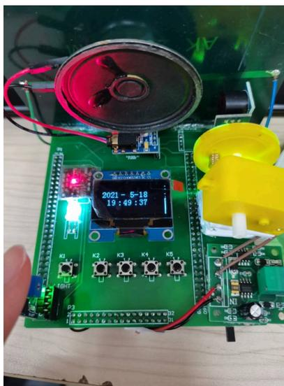
**Figure 14.** Turn on light test in case of dark.
