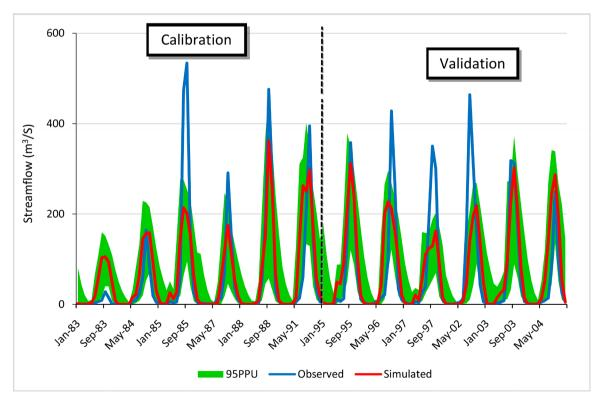
**Figure 3.** Observed and simulated hydrograph for the Marabadiassa station (left calibration period and right validation period).
