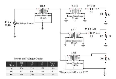
Figure 4. The scheme of converter 1 - 3 and simulations results.
