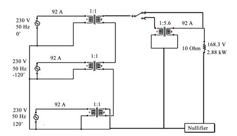
Figure 2. The scheme of converter 3 - 1 and simulations results.
